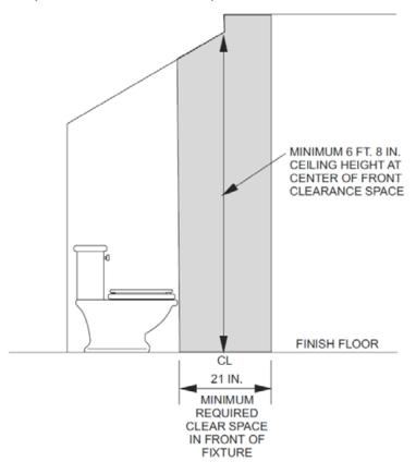
(tub). The clear space in front of the water closet shall be at least 21". Water closets must be sealed to the floor with appropriate caulks.
