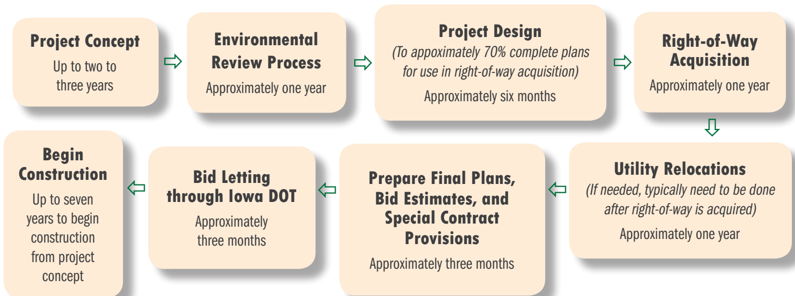
FIGURE 38: Flow Chart of a Typical Project Development Schedule After Funding is Received
